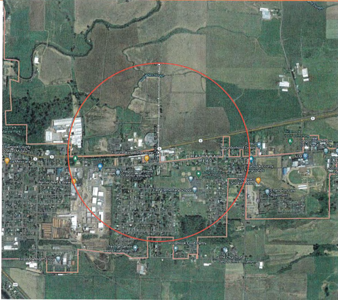
Figure showing Radius of 2600 ft surrounding site is categorized under Exposure C
