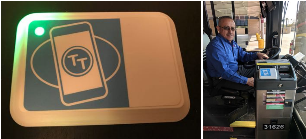
Standalone Token Transit Validators (left) and example Token Transit Validator on farebox (right)
