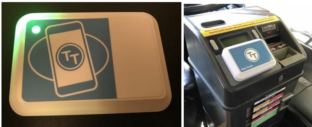
Standalone Token Transit Validators (left) and example Token Transit Validator on farebox (right). For reference, Token Transit validators are about the size of a deck of playing cards.
