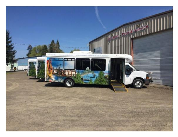
With these buses, we are beginning the transition of our fleet to low floor buses to make it easier for riders to get on and off of the buses without having to navigate stairs. With the loading ramp, we no longer have to have lifts on the buses to board passengers with mobility devices.
